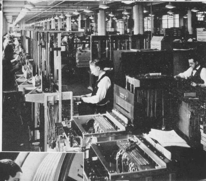
Standardization of switchboard design permits production of quality equipment by conveyorized methods.
