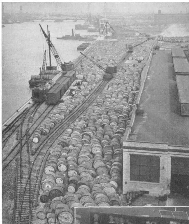
Kearny's cable yard, in which exchange area cable is stored against future orders. The normal stock is about 2,000 cable reels, ranging in weight from 1,600 to 6,500 pounds.
